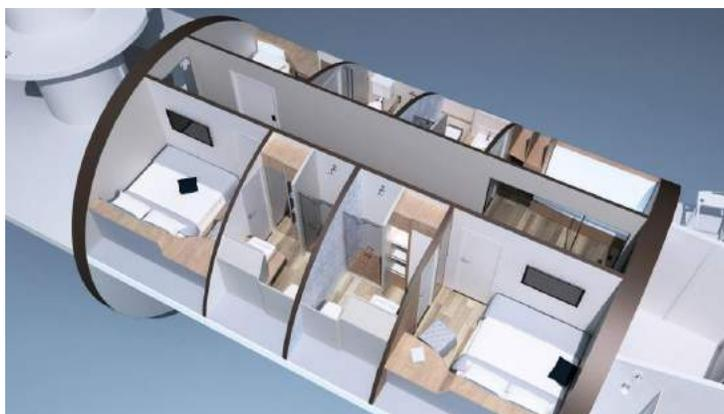
Carapace, which would be powered by a diesel-electric and fuel cell system, is designed to have a light aluminum superstructure that measures 256 feet in length.
